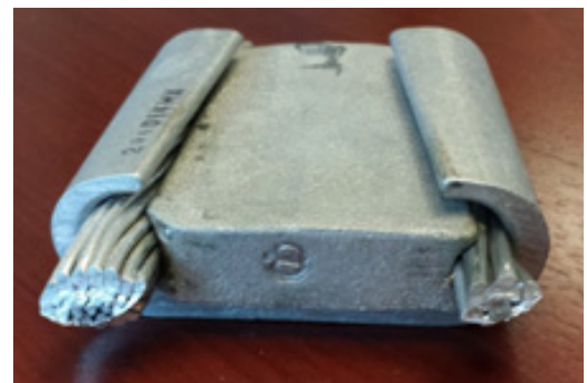
Figure 3.1-7 Manufacturer's mark embossed on end of wedge by installation tool
